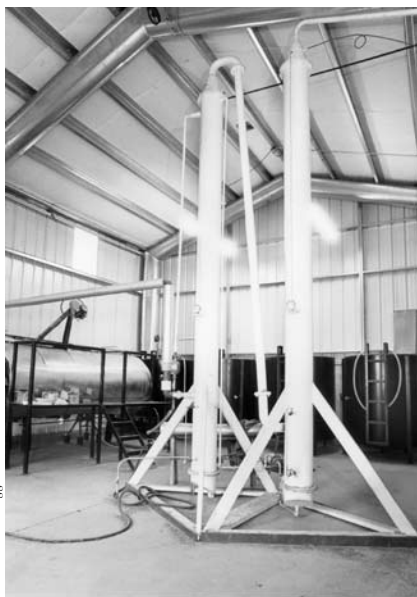
Jim Hall's self-built 12-inch continuous distillery. Mash cooker and grain auger are to the left. Fermentation tanks are in the back.
