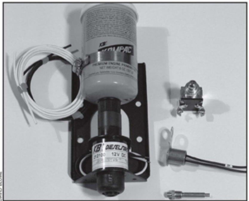
Fig. 17-4 Commercial ether start system. Although commercial systems are more expensive, they deliver a measured amount of ether, which more or less idiot-proofs the system against flooding the engine with explosive ether. On the right (from top to bottom) is a momentary contact switch for manually starting, a thermostatic switch to be attached under any bolt on the block, and a very nice atomizer to be threaded into a drilled and tapped hole in the manifold. The roll of tubing on the left is used to connect the valve to the atomizer.
