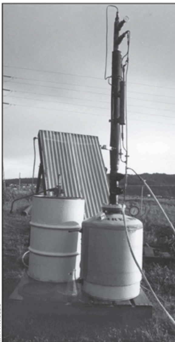
Fig. 8-14 Experimental solar vacuum still. Used by Wetlands Engineering and Technology for test batches. Heat energy comes from the panel in the rear.
