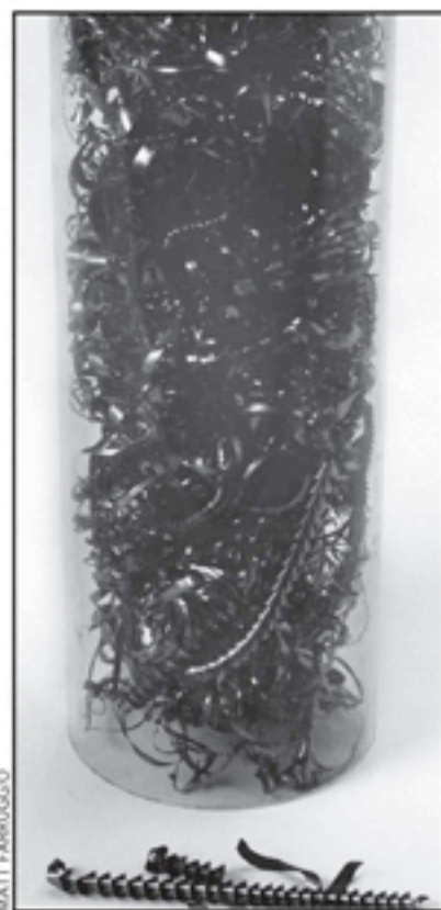
Fig. 9-15 Bronze wool packing. Far superior to marbles, bronze wool is okay to use in three-inch-diameter columns. In six-inch columns, the wool uses a lot more energy than pall rings to overcome greater back pressure, and the lower pads tend to load up with particles of mash in a pretty short time.
