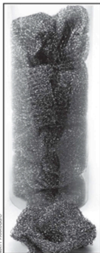
Fig. 9-15 Bronze wool packing. Far superior to marbles, bronze wool is okay to use in three-inch-diameter columns. In six-inch columns, the wool uses a lot more energy than pall rings to overcome greater back pressure, and the lower pads tend to load up with particles of mash in a pretty short time.
